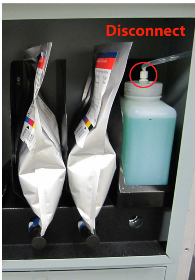
[98] Coolant Bottle is Located in the Primary Ink Bay
