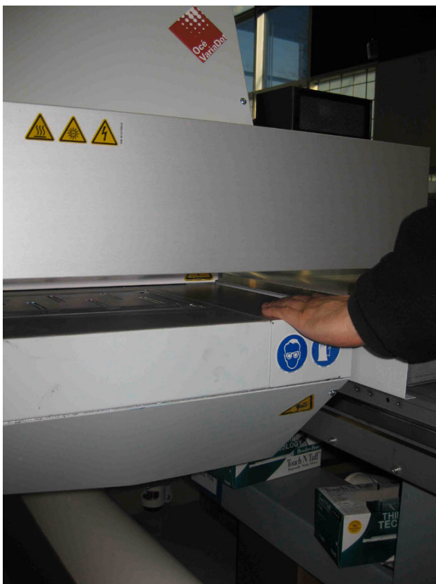
[5] Carriage Crush Hazard
