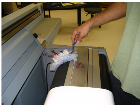
[105] Remove lint, dust, paper particles and debris
