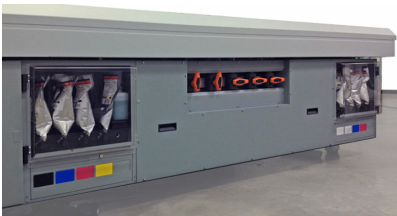
[23] Vacuum Zone Control Handles
