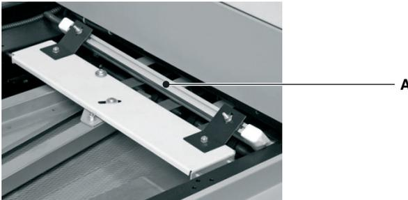
[49] The Static Elimination Bar in the Connecting Bridge
