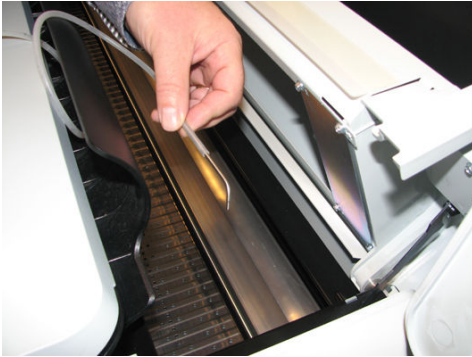
[244] Metal tube of ink filling tool
