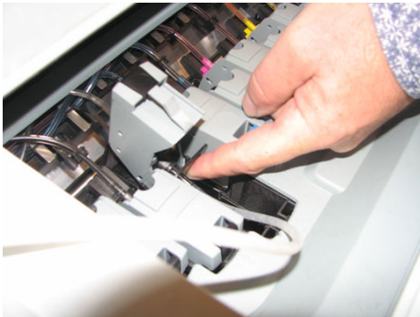
[247] Ink filling tool on empty ink tube
