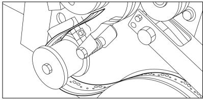
[77] Guiding the tape around the guide roller
