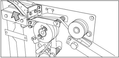
[86] Cutting the tape at the knife section
