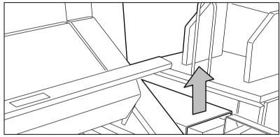
[113] Opening the top cover of the reinforcement unit
