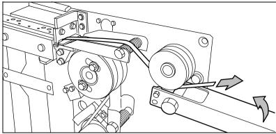
[84] Leading the protection sheet between the rollers
