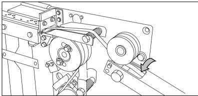
[85] Inserting the tape into the closed section of the slide
