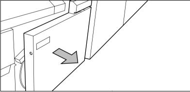
[115] Opening the front door of the reinforcement unit
