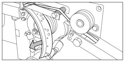
[75] Removing the trailing strip of the old tape
