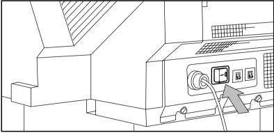
[6] On/off switch of the printer
