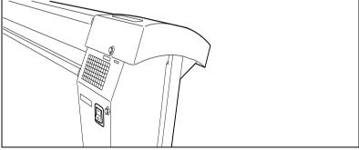
[10] On/off switch of the scanner
