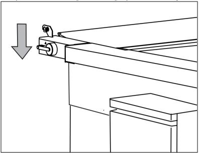
[121] To fold, switch the lever downward
