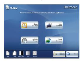
The **ShareScan Client** is installed on a ScanStation. It displays the user interface and handles user input. It passes all information, including the raw scanned image file, to the Services Manager for processing.
